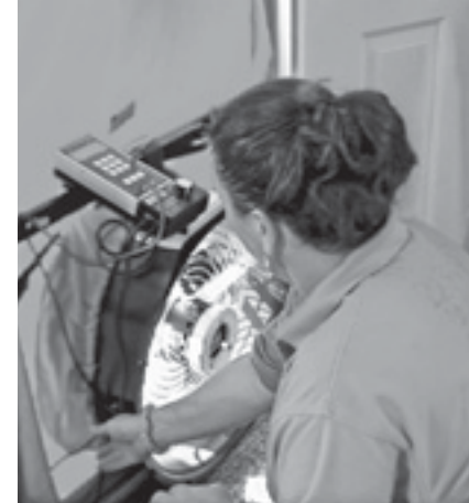
Blower door test to assess airflow.
