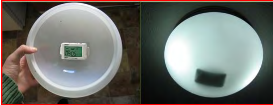
Logger is too visible to homeowner.
