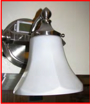
Logger is placed so the fixture blocks it from detecting light.
