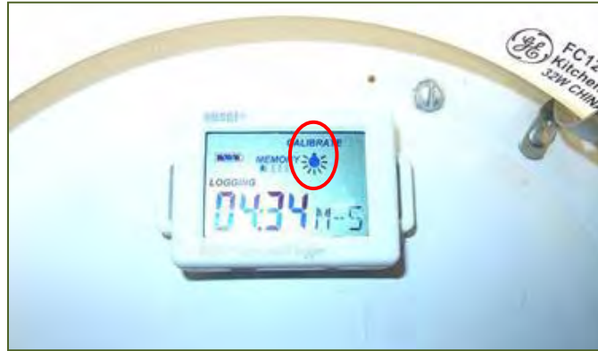
Figure 6: Light On - Bulb On
