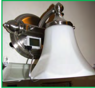
Logger is placed next to the fixture with a light pipe curving around fixture to focus directly on the light source
