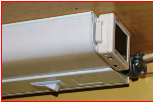
Logger is installed away from the light source and the light sensor is up against the cabinet.
