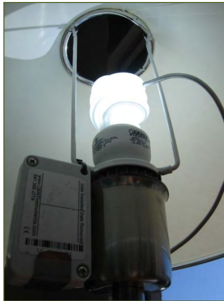
Figure 2: Fiber Optic Eye Aimed at Brightest Part of Light
