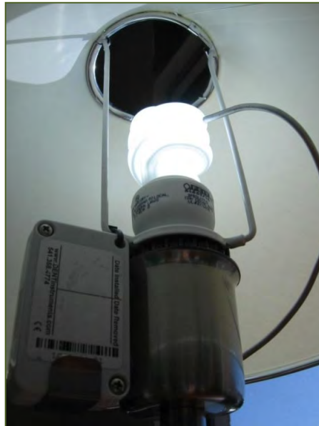
Figure 5: Fiber Optic Eye Aimed at Brightest Part of Light
