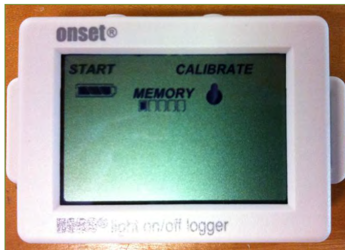
Figure 7: Logger Screen after 10 Minutes
