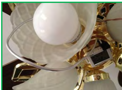
If unable to place the logger closer, use light pipe to focus in on light source
