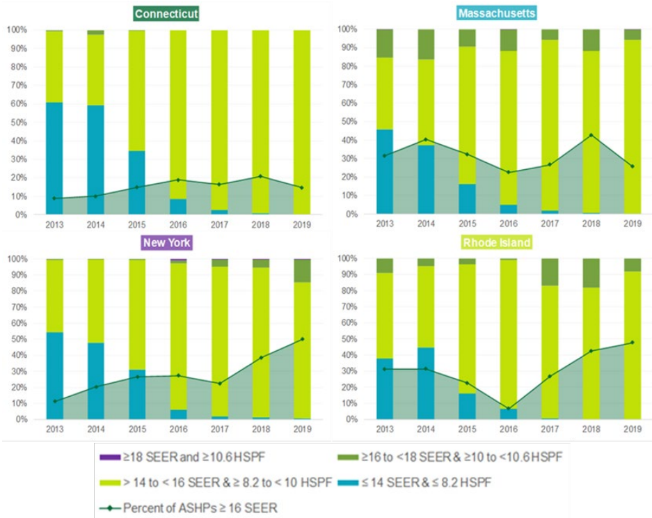
Figure 22: ASHP Installations by Efficiency (SEER and HSPF) and State, HARDI
