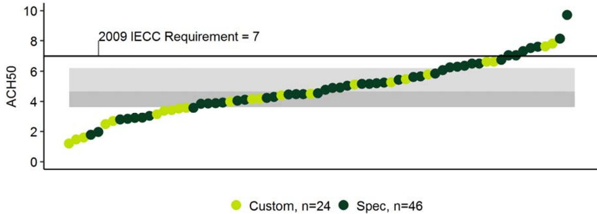
Figure 23: Air Infiltration (ACH50)
