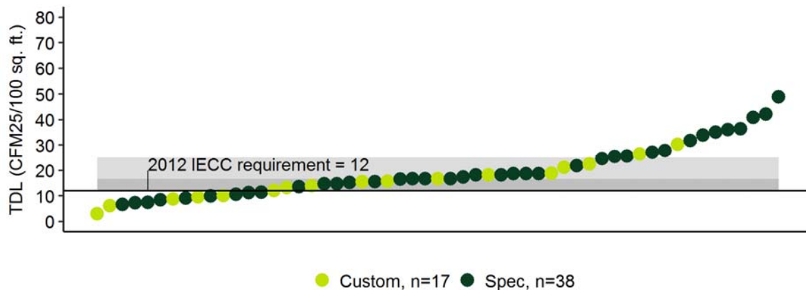
Figure 22: Total Duct Leakage
