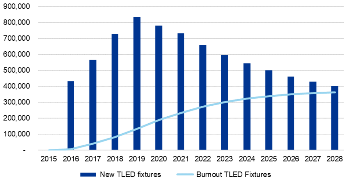
Figure 3-1. Total number of new TLED fixtures installed compared to rate of TLED fixture burnout
